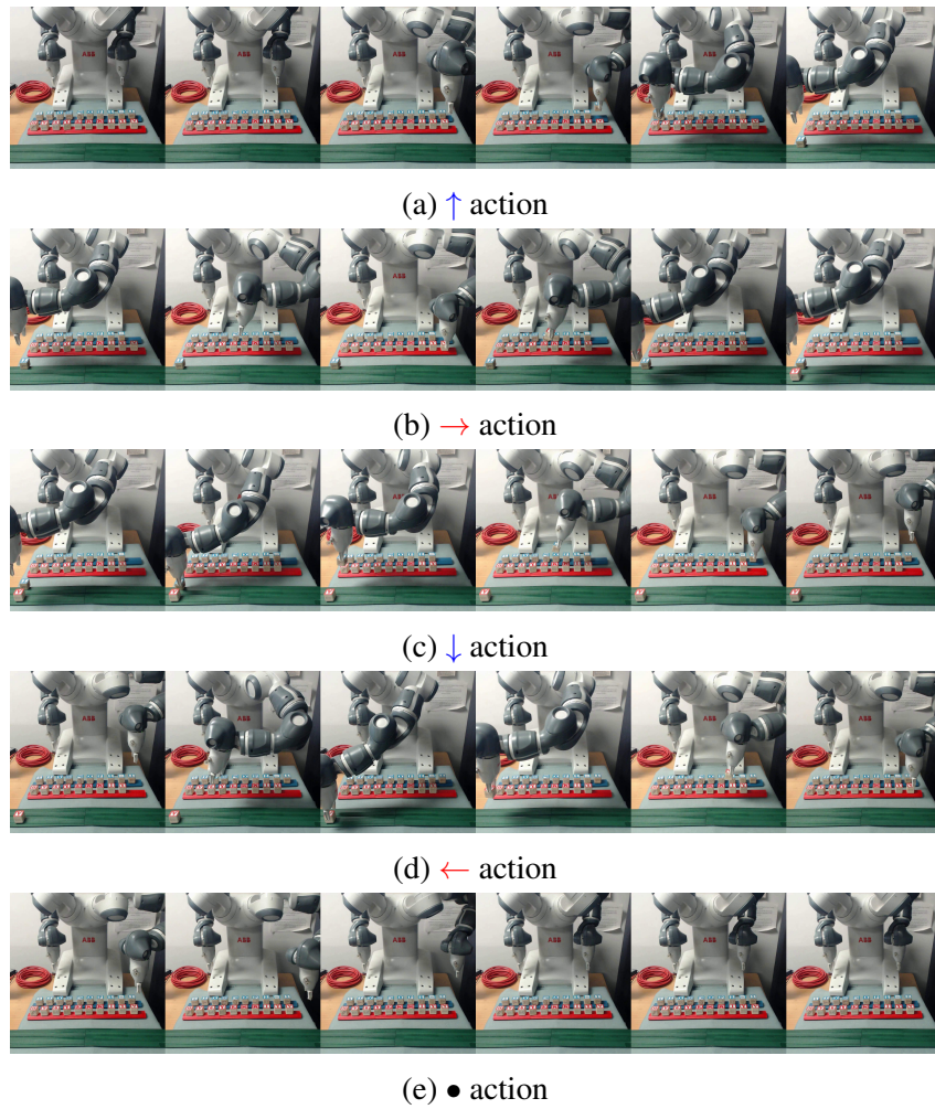
Figure 3.2: Sample robot arm trajectories for each action in the bin packing domain.
